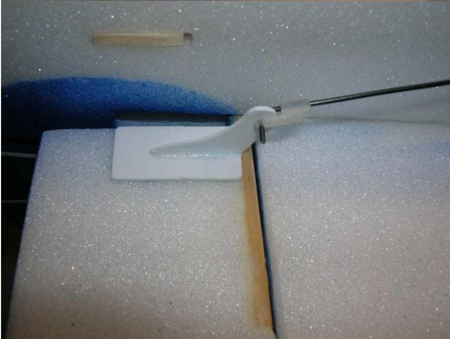
**Install the 1/32" diameter wire elevator push rod securing it at the servo end with a Dubro Mini E/Z Connector, and at the control horn end with a Dubro E/Z Link.**
